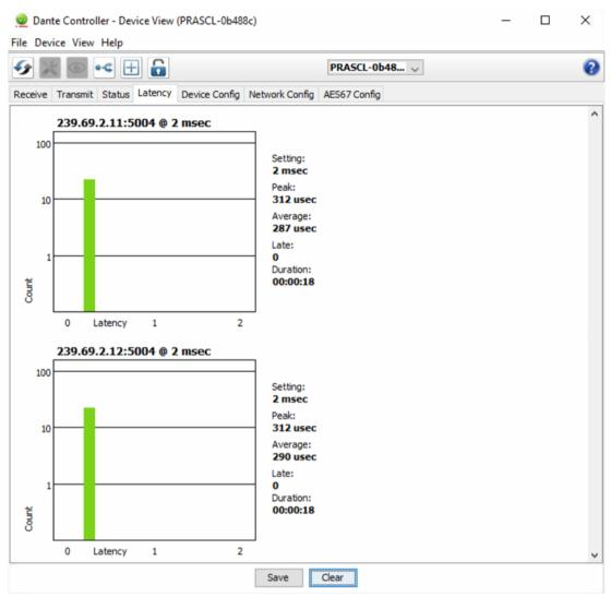
The latency scattered around it could be caused by an improperly configured switch in the path between the PRA-APAS and PRAESENSA or between the clock master.
