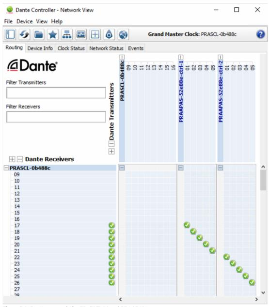
Figure 5.3: Routing example for PRAESENSA and PRA-APAS system
